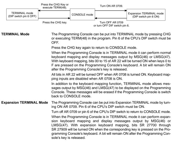
All bits from SR 27700 through SR 27909 will be turned OFF when AR 0708 is turned ON. Expansion keyboard mapping inputs are disabled when AR 0708 is ON.
